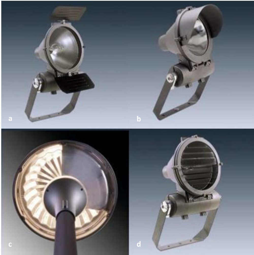
Figure 6.5. Luminaire accessories to direct light: (a) shield “barn doors”; (b) cowl (hood); (c) shield; and (d) external louvre. Images from Philips and Thorn (ILP 2011)
