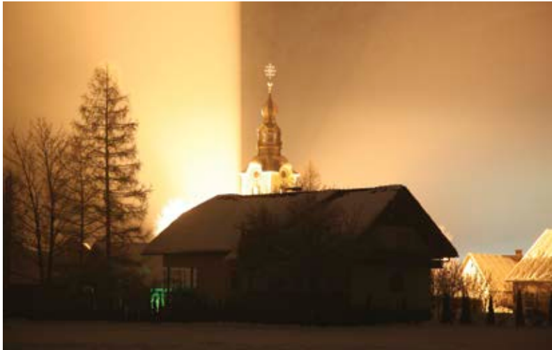
A smaller country church. The photograph was taken in clear weather with somewhat increased air humidity as is usual at night. The photo clearly shows light beams that miss the belfry and illuminate the sky.
